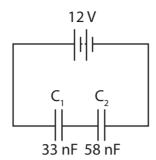
**17** (a) Calculate the total capacitance in the circuit.
