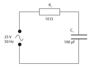
**19** Calculate the total impedance in the circuit.
